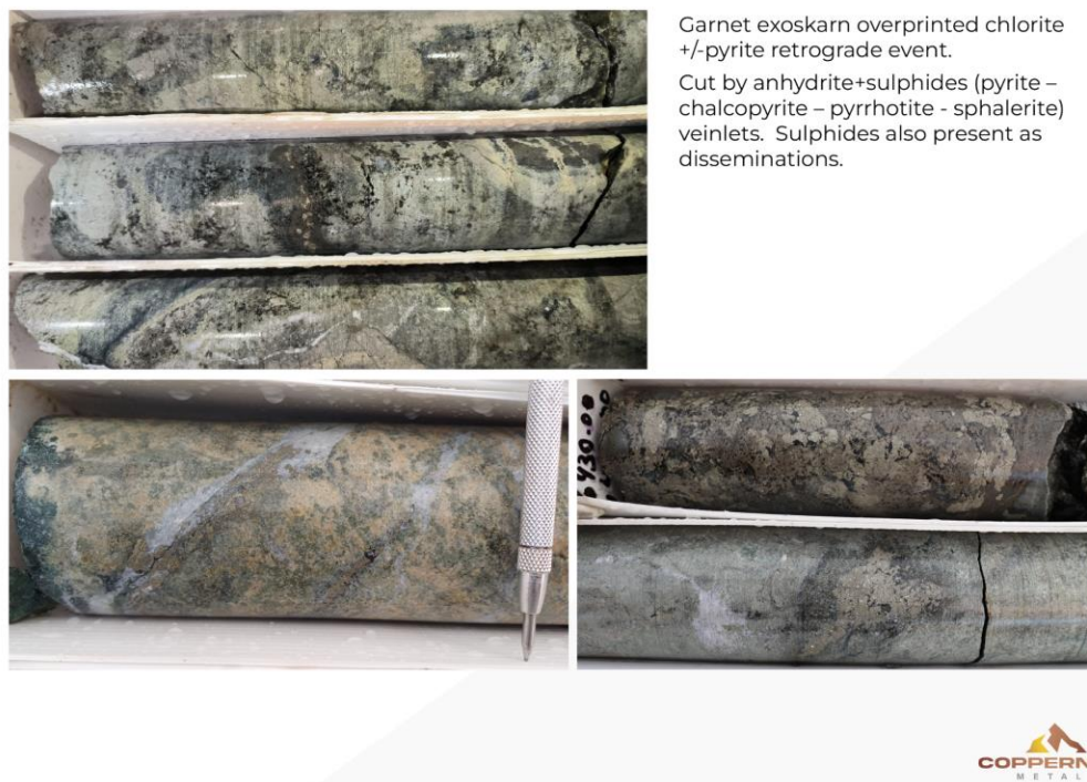
Figure 5 - Zones with high concentrations of sulphide minerals including pyrite, chalcopyrite and pyrrhotite in fourth hole
